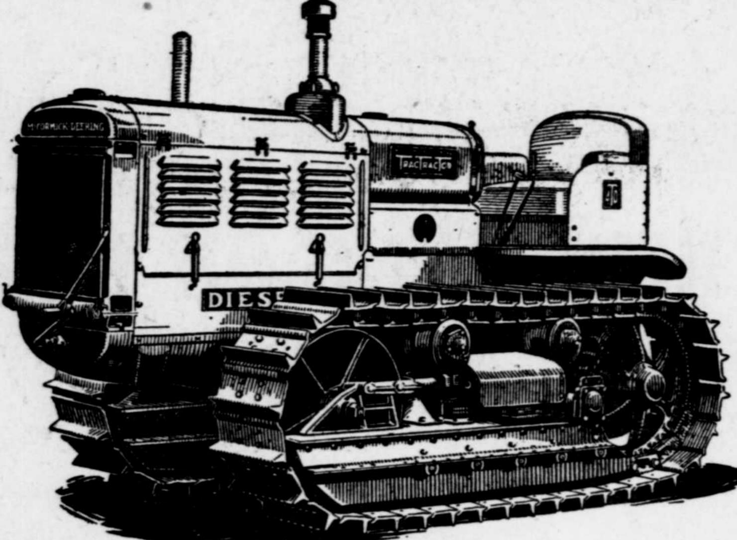
TERE is good news for crawler tractor users who need heavy-duty performance at the lowest possible cost per hour. International Harvester engineers have adapted the Diesel principle to TracTracTor operation. No auxiliary engine of any kind is used. The International Harvester Diesel engine is characterized by remarkable ease of starting and quick conversion to low-grade fuel. In fact, the shift from gasoline to Diesel fuel is almost entirely automatic.
