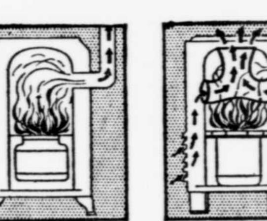
TURNS WASTE INTO WARMTH! Ordinary heater (left) allows much heat to escape up the flue. Unique Intensi-Fire Air Duct (right), found only in the Estate Oil Heatrola, blocks heat - sends it into rooms.
